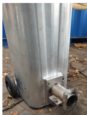
Mounting the ash auger. Positioning and mounting the ash bin. Fig 11
