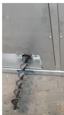
Mounting the ash auger. Positioning and mounting the ash bin. Fig 11
