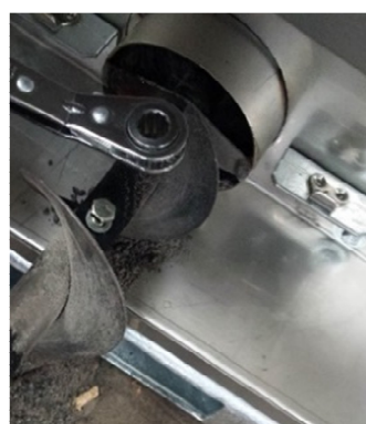
Mounting the ash auger. Positioning and mounting the ash bin. Fig 11
